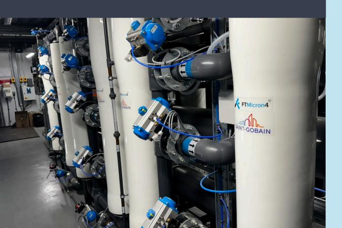
**Microfiltration** is a physical filtration process where a contaminated fluid passes through a specific pore sized membrane to separate out microorganisms and suspended particles.
